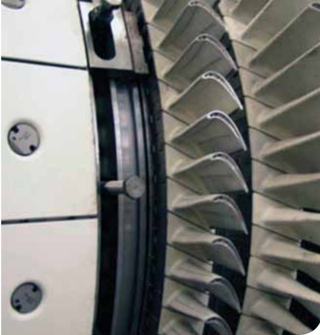
AE64.3A Gas Turbine combustion chamber tiles and turbine blades
