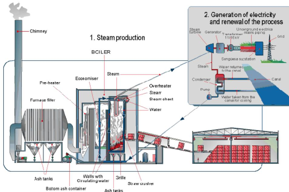
Figure 1: Process diagram
