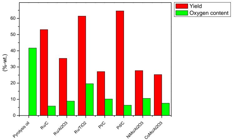
Catalyst screening in semi-Batch system at 350 °C and 200 bar of H<sub>2</sub> for 4h.
