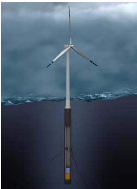
Figure 5.2: The floating wind turbine concept Hywind. Source: Norwegian Hydro and Solberg production
