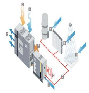
1) Cold water 2) Compressed air 3) Electric power 4) Air 5) Oil circuit 6) Energy recovery 7) Warm water Diagram credit: Atlas Copco
