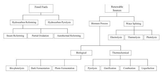
Figure 3. A breakdown of hydrogen production methods (reproduced from (Nikolaidis and Poullikkas 2017)). With the exception of biological processes, all other methods produce medium to high temperature process heat. Page 8 of 40 Version B
