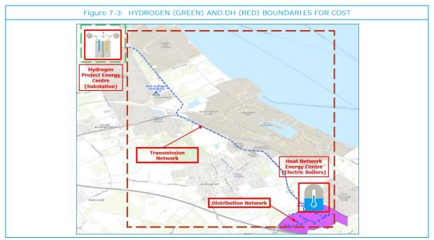
It was assumed that the cost for the waste heat recovery substation and its associated energy centre investment and running costs are in the scope of hydrogen project. The transmission network, DHN energy centre and the distribution heat network was considered to be in the scope of the DHN project.
