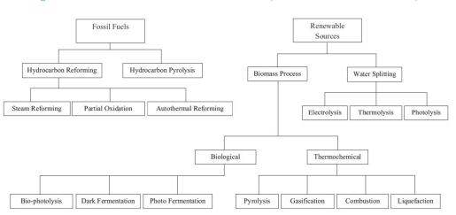
Figure 2-1: HYDROGEN PRODUCTION PROCESSES (Nikolaidis and Poullikkas 2017)
