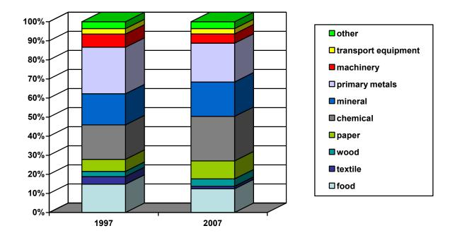
Figure 13. Energy consumption in manufacturing by branch
