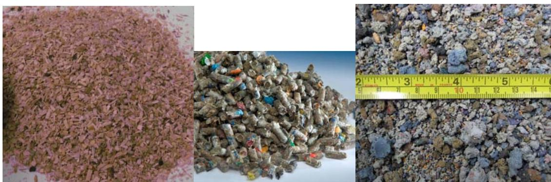
Figure 3.1 Test fuels, from left to right: beech wood chips, Rofire pellets and industrial waste.
