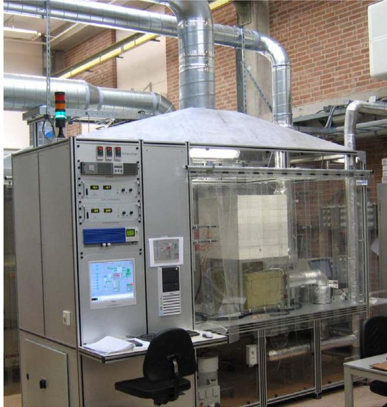
Figure 2.7 *SOFC test facility with load unit and computer (left), furnace with gas pre-heaters (centre), fuel gas supply (right) and off-gas ducts (top).*
