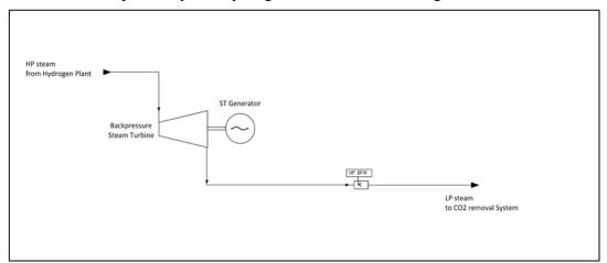
The high pressure steam is expanded in the steam turbine to produce electricity and generates the low pressure steam (at 0.44 MPa and 177°C). The LP steam is then sent to the Stripper's Reboiler with a small part being fed to the deaerator (as supplementary steam for stripping).
