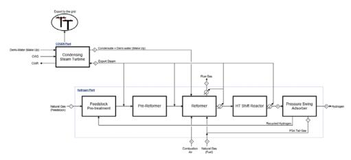
Figure 1: Base Case - SMR plant without CO<sub>2</sub> capture producing 100,000 Nm<sup>3</sup>/h H<sub>2</sub>.
