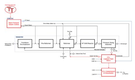
Figure 4: Case 2A - SMR plant with capture of CO<sub>2</sub> from PSA tail gas using MDEA
