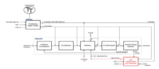
Figure 5: Case 2B - SMR Plant with capture of CO<sub>2</sub> from PSA tail gas using low temperature and membrane separation
