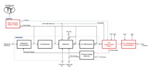
Figure 2: Case 1A - SMR Plant with capture of CO<sub>2</sub> from shifted syngas using MDEA
