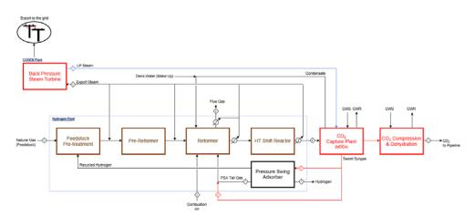
Figure 3: Case 1B - SMR Plant with H<sub>2</sub> rich burners and capture of CO<sub>2</sub> from shifted syngas using MDEA
