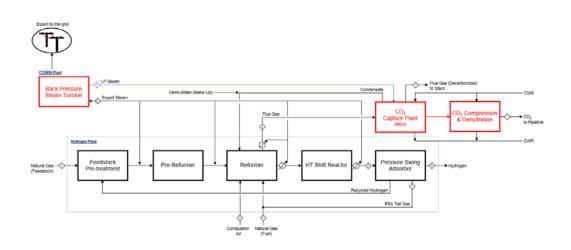
Figure 6: Case 3 - SMR Plant with capture of CO<sub>2</sub> from SMR flue gas using MEA
