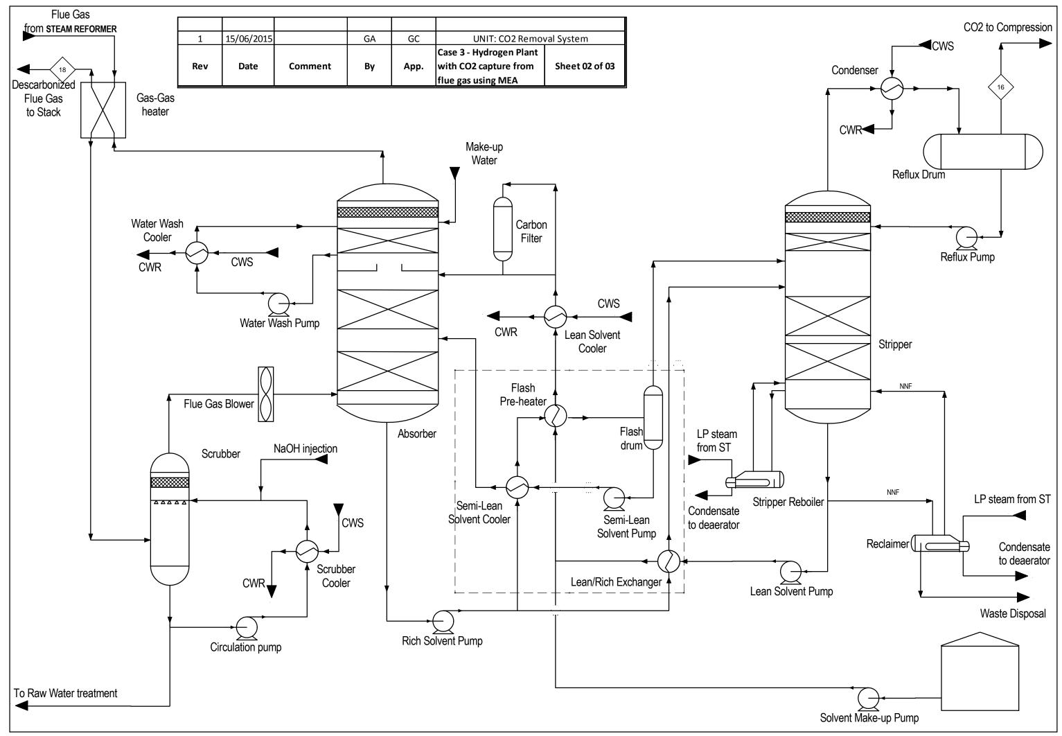
The BFD above is a simplified representation of a Post combustion CO2 removal system. Equipment shown within the dotted line and relevant configuration may change depending on Licensor Technology
