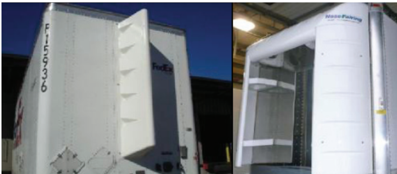
FIGURE 5-13 Laydon vortex stabilizer (left) and nose fairing (right). SOURCE: Courtesy of Laydon Composites.
