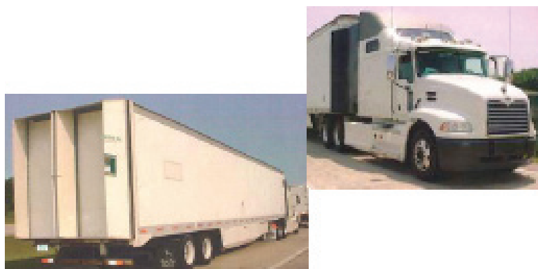
FIGURE 5-25 Mack truck with aerodynamic device combination. SOURCE: TMA (2007), pp. 57, 58, 60.
