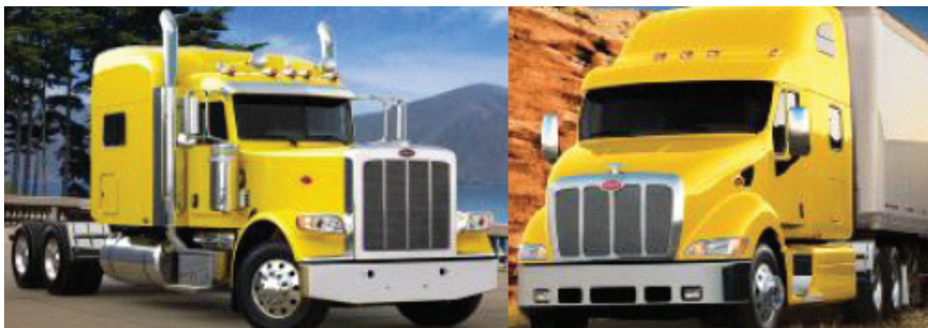
FIGURE 5-10 Peterbilt Traditional Model 389 (left) and Aerodynamic Model 387 2 (right) (SmartWay). SOURCE: Courtesy of Peterbilt Motors Company.
