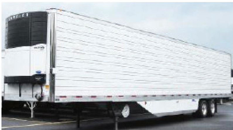
FIGURE 5-18 Refrigerated van trailer with Freight Wing skirts. SOURCE: Courtesy of Freight Wing.
