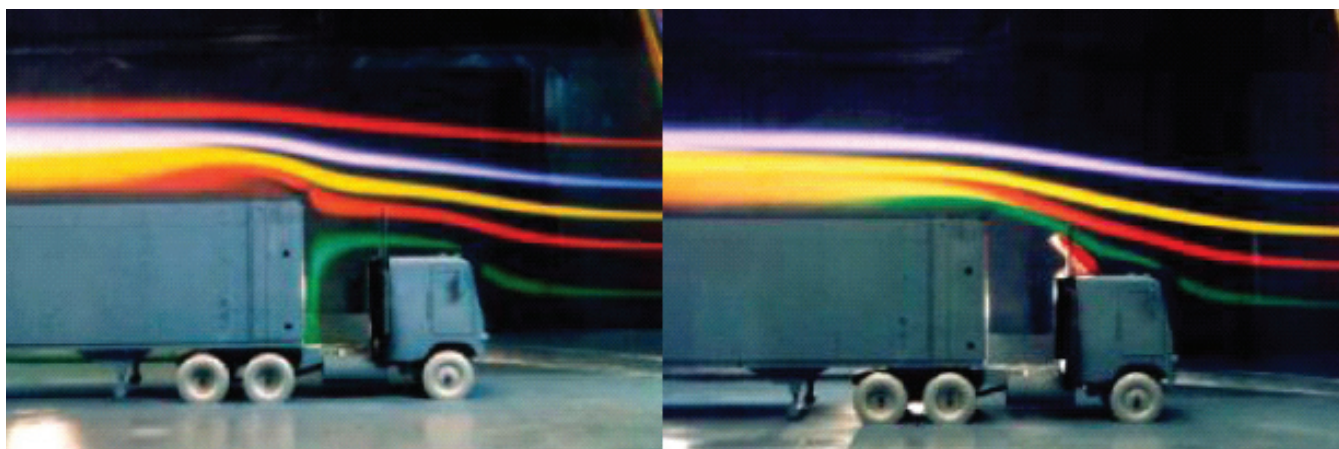
FIGURE 5-3 National Research Council of Canada: Smoke pictures, cab with deflector (right). SOURCE: Cooper (2004), p. 11, Fig. 2. Reprinted with kind permission of Springer Science and Business Media.
