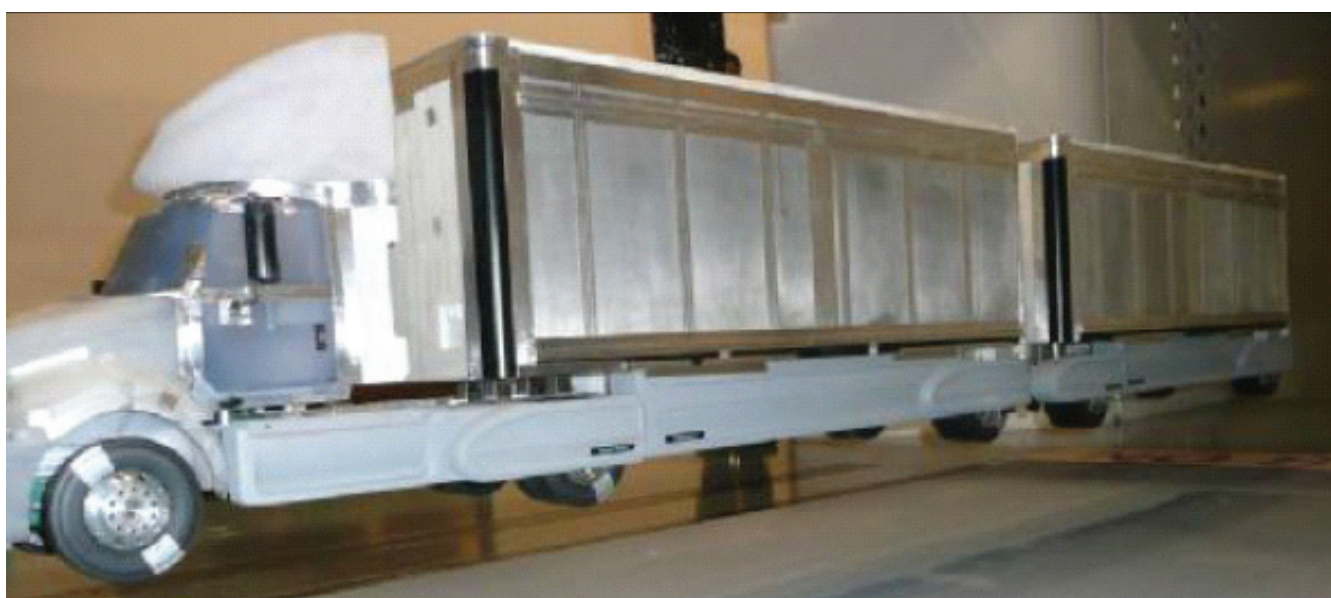
FIGURE 5-17 Laydon double trailer arrangement with trailer skirts and vortex stabilizers on both trailers; SOURCE: Courtesy of Laydon Composites.
