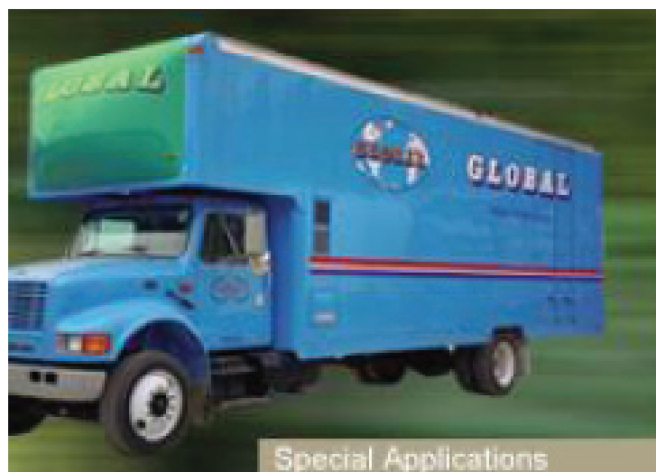
FIGURE 5-26 Nose Cone fairing on face of straight truck. SOURCE: Photo provided with permission by FitzGerald Corporation, national marketer for Nose Cone Mfg. Co. Nose Cone is a registered trademark.
