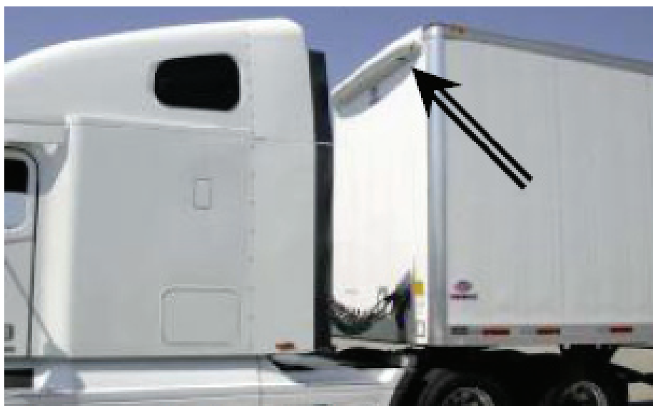
FIGURE 5-12 Nose cone trailer “eyebrow.” SOURCE: Photo provided with permission by FitzGerald Corporation, national marketer for Nose Cone Mfg. Co. Nose Cone is a registered trademark.
