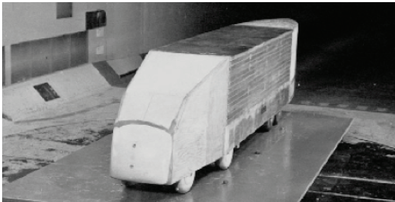
FIGURE 5-2 University of Maryland, streamlined tractor, closed gap, three-quarter trailer skirt, full boat tail. SOURCE: Cooper (2004), p. 15, Fig. 4, Case 8. Reprinted with kind permission of Springer Science and Business Media.
