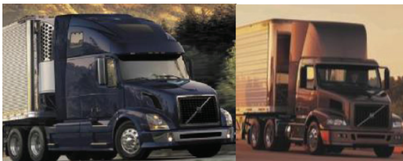
FIGURE 5-9 Volvo full sleeper cab (left) and day cab (right). SOURCE: Courtesy of Volvo.
