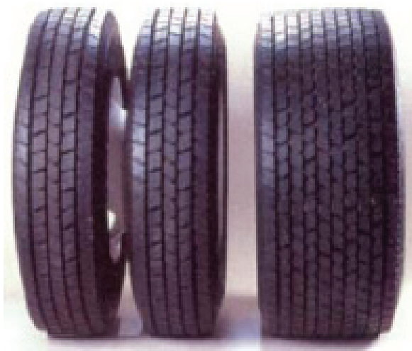
FIGURE 5-29 New-generation wide-base single tire (right) to reduce the rolling resistance of conventional dual tires (left). SOURCE: Presentation to the committee by C. Bradley and S. Nelson, Michelin Tire North America, "Truck Tires and Rolling Resistance," February 4, 2009. Courtesy of Michelin Tire North America.
