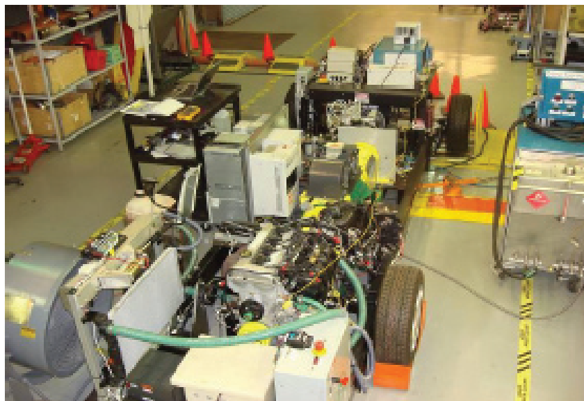
FIGURE H-13 Mixing components hardware and software—MATT example. SOURCE: Argonne National Laboratory.
