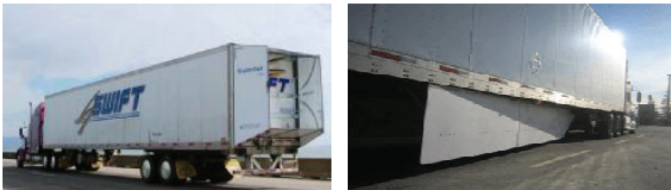
FIGURE 5-11 ATDynamics trailer tail (left) and FreightWing trailer skirt (right). SOURCE: Courtesy of Freight Wing.
