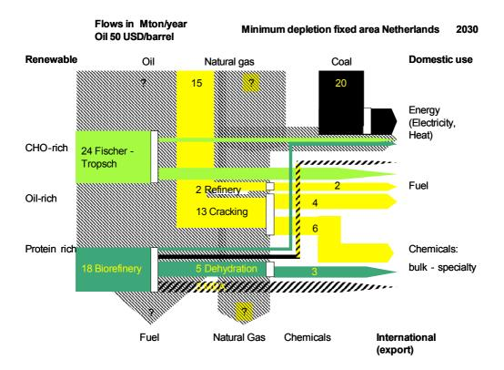
Figure 13 Calculated mass flows for the preferred processes for minimum depletion on restricted area as optimisation criterion (Case 4).
