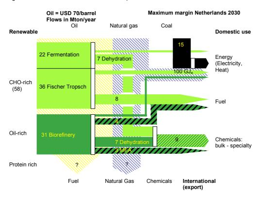
Figure 17 At an oil price of 70 USD/barrel, a maximum margin scenario proposes the production of chemicals and fuels from 100% biomass
