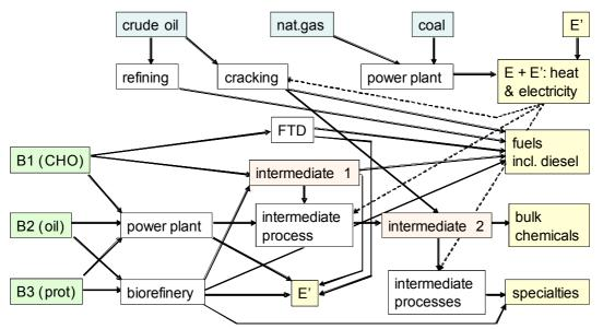
**Figure S1**. Schematic overview of the simplified Dutch energy situation, converting renewable and fossil feedstocks into desired product classes. B1 corresponds to carbohydrate-rich biomass, B2 to oil-rich biomass and B3 to protein-rich biomass. For reasons of overview, (co)produced electricity has been marked as *E*'.
