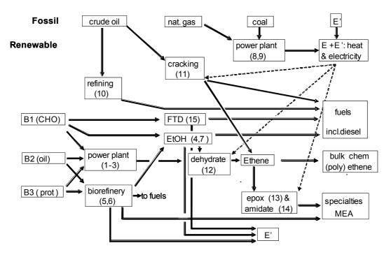
**Figure 7**. Schematic overview of the lumped processes, converting the renewable and fossil feedstocks into desired product classes.
