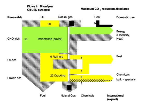
Figure 14 Mass flows for the preferred processes for maximum CO<sub>2</sub> emission reduction and a fixed area as optimisation criterion (Case 5).
