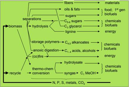
Figure 6 Schematical and simplified overview of fractionation and conversion of biomass in desired industrial and consumer products.
