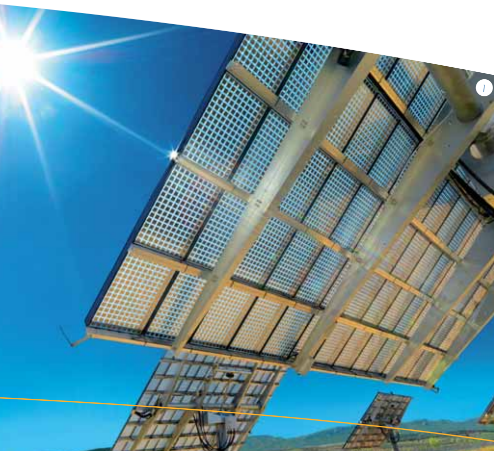
1. CPV systems produced by Soitec Solar. These modules with Concentrix™ technology use Fresnel lenses to concentrate sunlight 500 times onto cells of 2 mm diameter. ©SOITEC SOLAR
