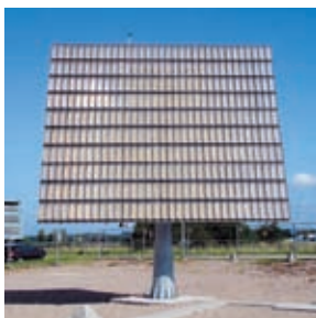
A module produced by Concentrix Solar, which uses Fresnel lenses to concentrate sunlight 500 times onto cells of 2mm diameter Source : Fraunhofer ISE
