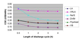
Fig. 3. Added cost (COE) vs. discharge time, 2.5 MW T&D application operating 250 d/year.
