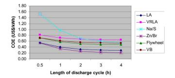
Fig. 4. Added cost (COE) vs. discharge time, 2.5 MW T&D application operating 100 d/year.
