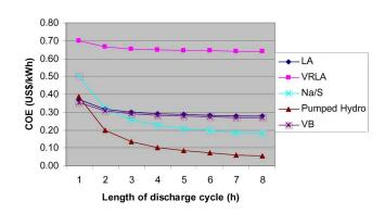
Fig. 1. Added cost (COE) vs. discharge time, 10 MW generation application operating 250 d/year.
